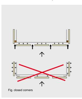
If certain conditions are met, the pressure coefficient ( $c_{pe}$ ) decreases, resulting in a lower windload. Pressure equalization is specified in Eurocode EN 1991-1-4, with further details in the National Annex.
